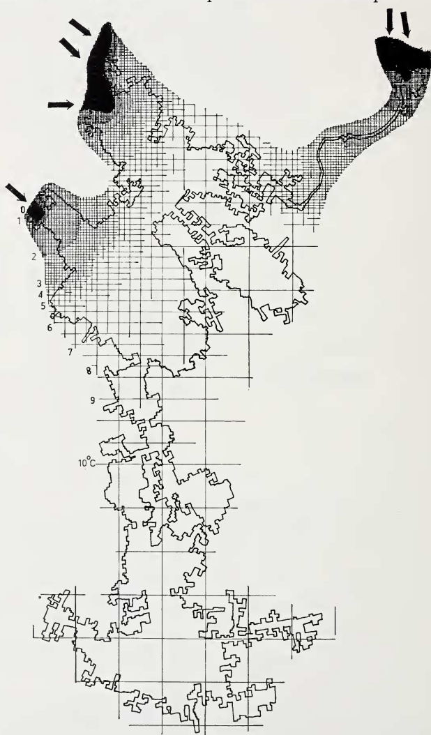
Fig. 2. Distribution of roof air temperatures on February 28, 1963. Outside temperature around freezing point ( -0,2^{\circ}\text{C} )
